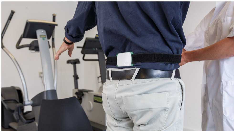
Fig 2. The test leaders attaches the measurement device. The device includes 3 accelerometers and 3 gyroscopes and has a wireless connection to the remote control of the test leader and the supporting computer with software controlling the test protocol.
